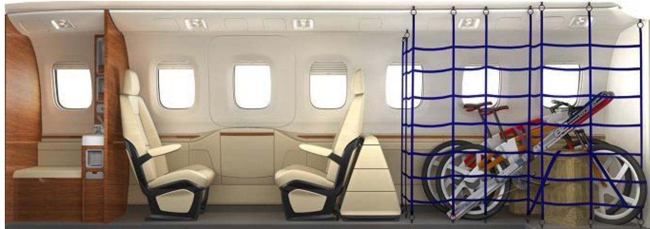
Quick removal – plug and play concept means removal of seats in 1/2 hour
