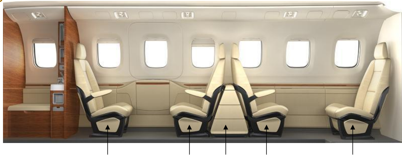
Quick removal – plug and play concept means removal of seats in 1/2 hour
