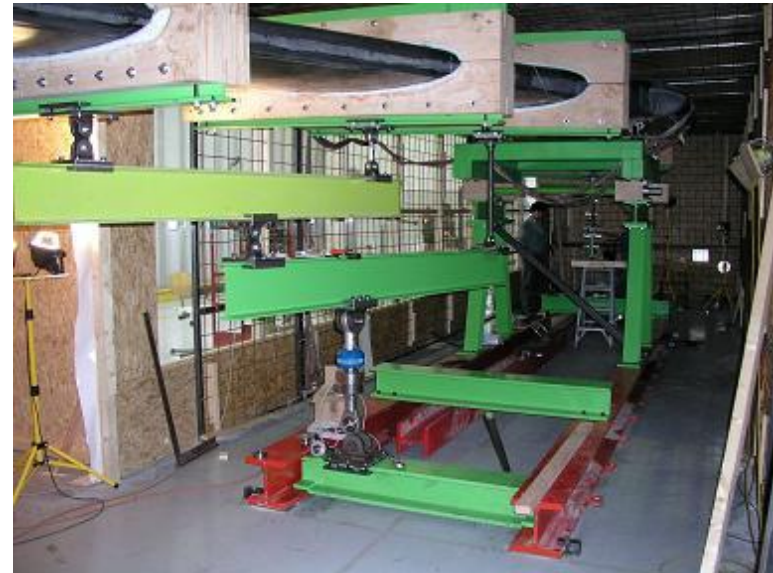
Wing static test
