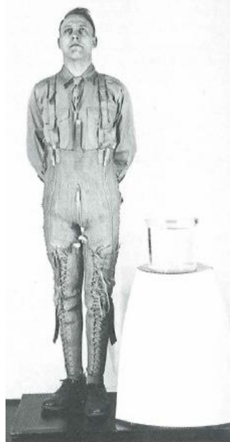
Figure 5. Frank's Flying Suit 1940s prototype of a fluid-filled G protection garment.
