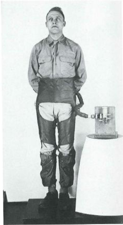
Figure 2. 1940s Prototype of a Pneumatic G Suit
