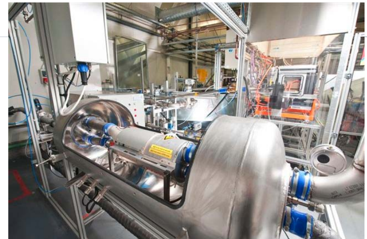
Inert Gas Conditioning System
